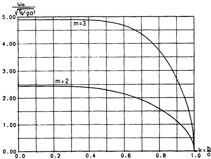
Fig. 2. Uncoupled liquid frequency for frictionless liquid.
