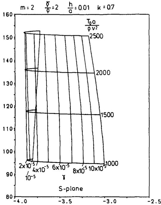
Fig. 6. Coupled liquid frequency in S plane.
